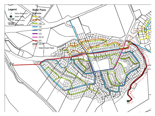
A 150mm water main was extended to the Stalker Road roundabout and across the highway in early 2016. This main exists in stalker Road adjoining the subject site. The static water pressure in the pipe varies from approx. 350kPa at the Oxfordshire Intersection down to 150kPa at the State Highway intersection given its relative elevation to the Shotover Country water reservoir.
