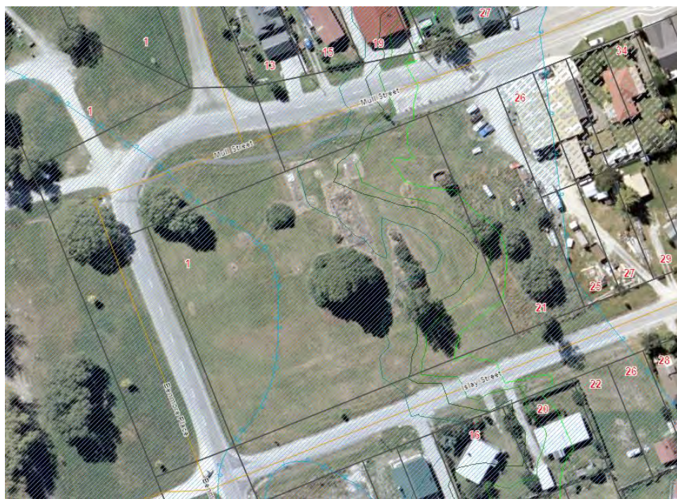
Figure 3: Showing Flood Contours (150, 100, 75 and 50 year return period events) and Extent of Flooding (blue hatched area)
