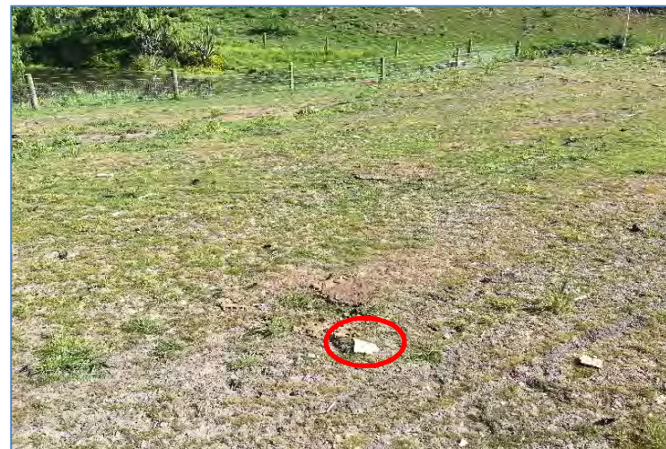
Photo 6: Potentially asbestos-containing cement fibre board fragment. on building platform.
