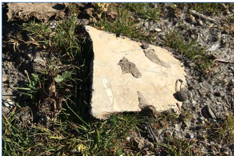
Photo 5: Potentially asbestos-containing cement fibre board fragment.
