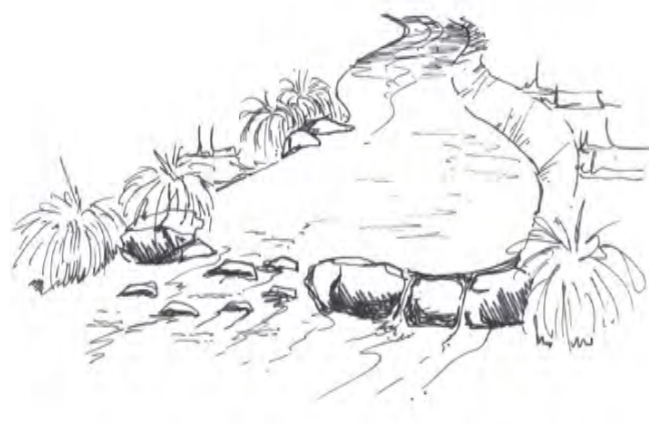
Creek channel with rock weir to flood the natural creek bed contours and riffles to allow fish passage
