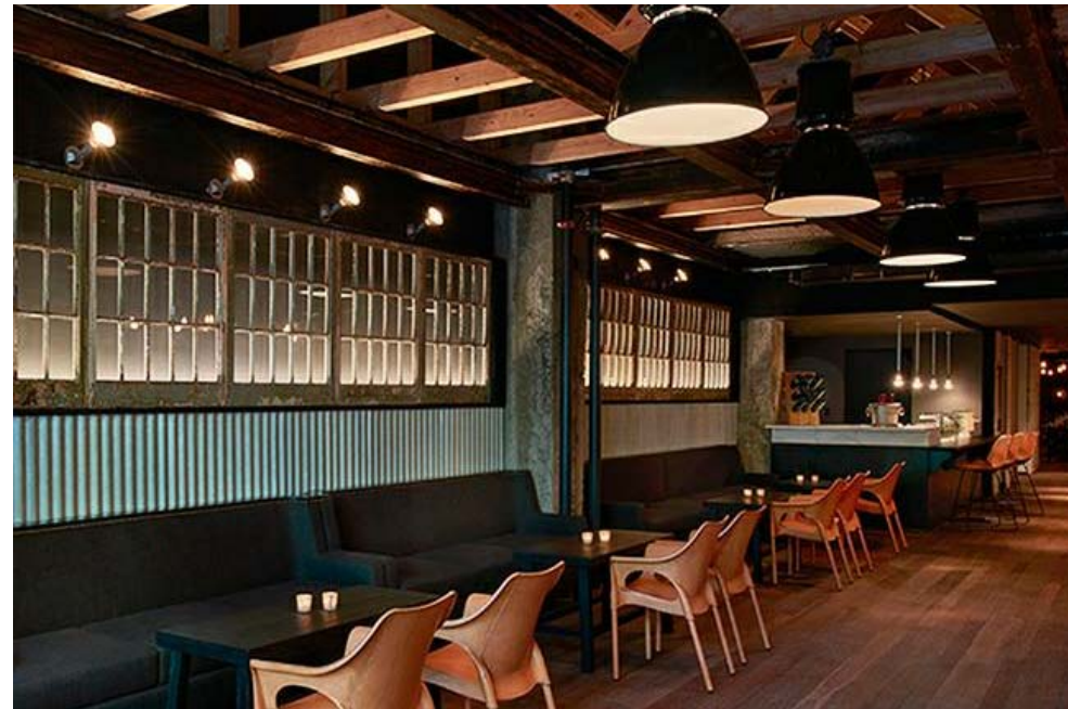
Precedent Image for lighting to the first floor dining area. Note uplighting to timber roof framing
