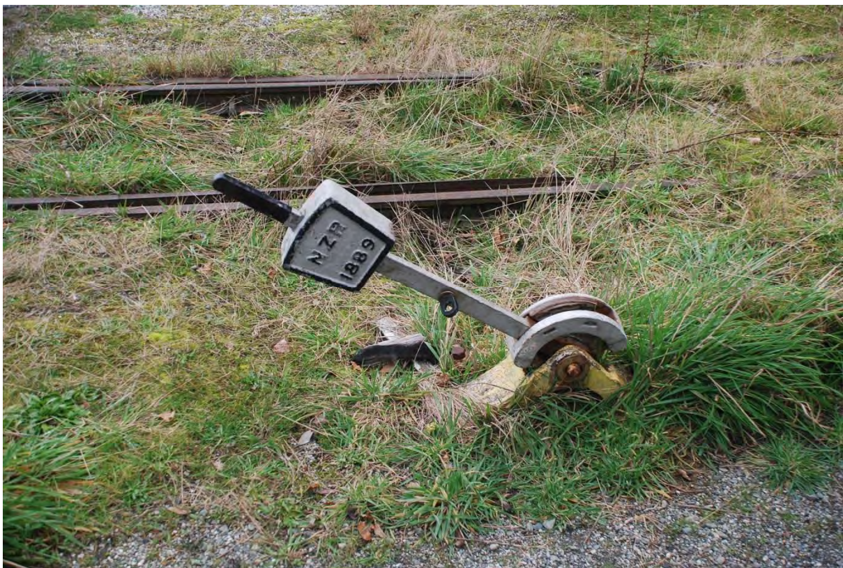
Photo 4 A points lever between the wharf shed and the station with the inscription 'NZR 1889'
