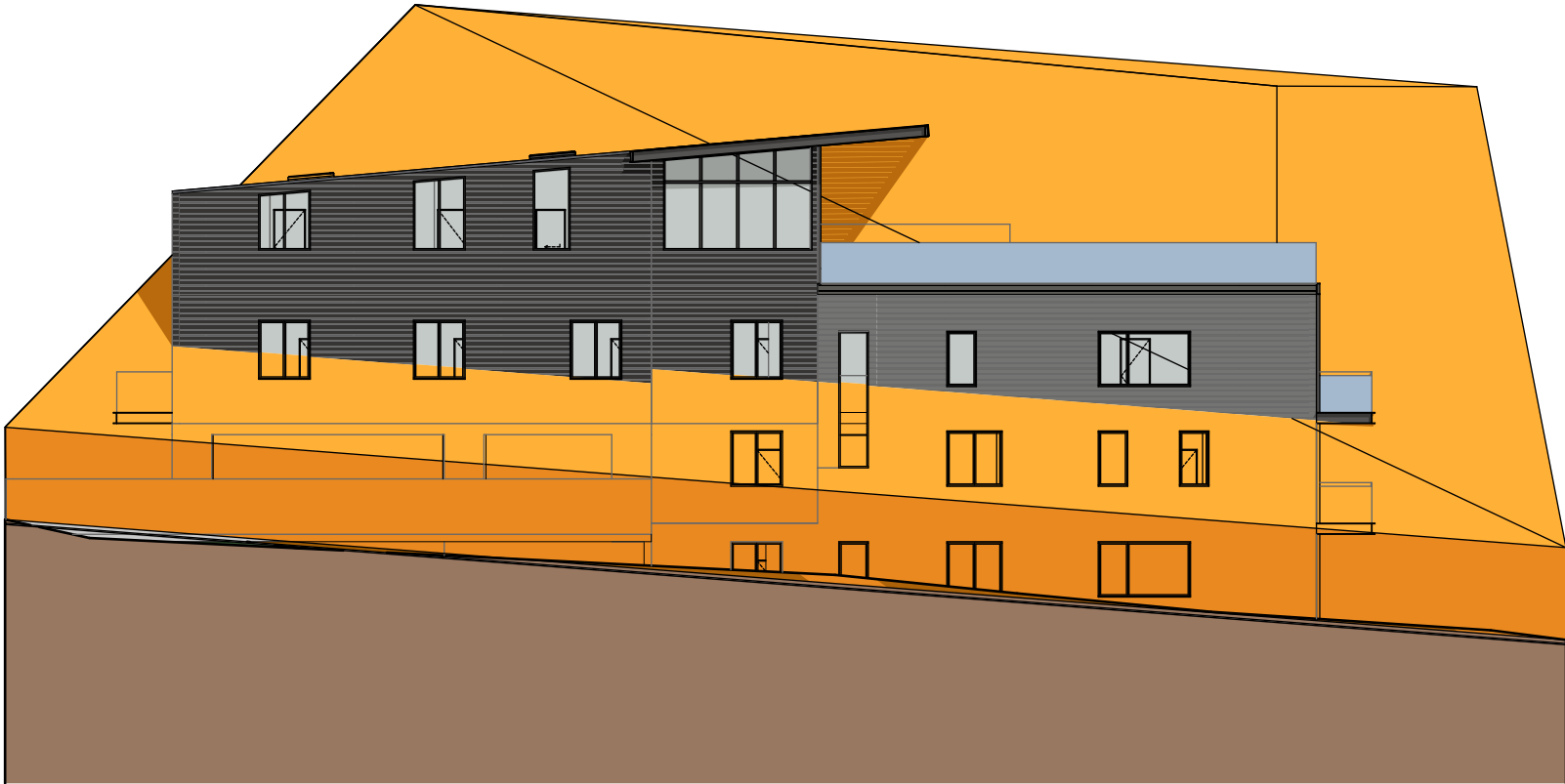
15m Height Limit Elevation 1:200
