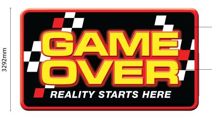
Digital Print Applied to 4.5 ACM Panels. Screw fixed to Exterior Cladding Silicon sealed
